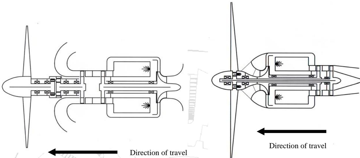
Considerable care must be taken when installing the back to back arrangement of engine, as it is necessary to avoid the hot exhaust gases from being re-ingested by the intake. Re-ingestion will result in the engine overheating with an associated risk of fire. No such risk affects the concentric arrangement but means must be found of safely ducting the hot gasses from the exhaust, if the engine is mounted in an enclosed fuselage.
