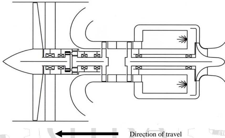
Considerable care must be taken when installing this arrangement of engine, as it is necessary to avoid the hot exhaust gases being re-ingested by the intake.
