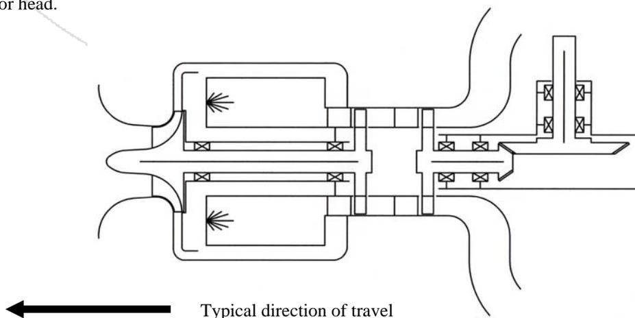
For clarity, the diagram above shows the exhaust and the output shaft being on the same plane. However, in practice, the exhaust and output shaft are typically arranged 90 degs to each other.
